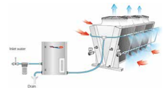
Fig. 3 Schematic for the ChillBooster™ showing how the high ambient temperature air is cooled by water droplets before passing over the coil.
